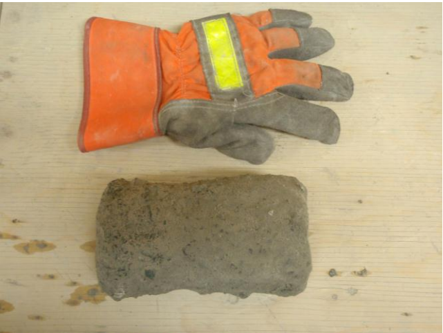
Photo 5: Drilled core HB12-ND-CORE-DC30-QA-201202010. Some drill chatter wore on the sides of the sample.
