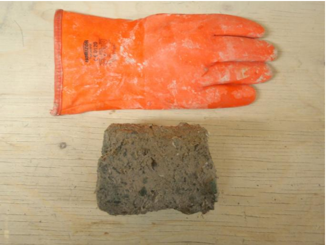
Photo 6: Drilled core HB12-ND-CORE-DC31-QA-201202010. Some gravel stuck in the annulus prompted a premature removal of this core.
