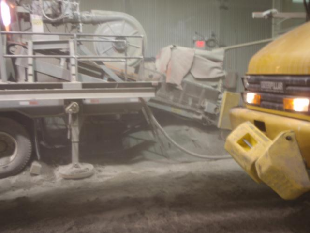
Photo 4: Material escaping from the feed belt at the frozen core plant
